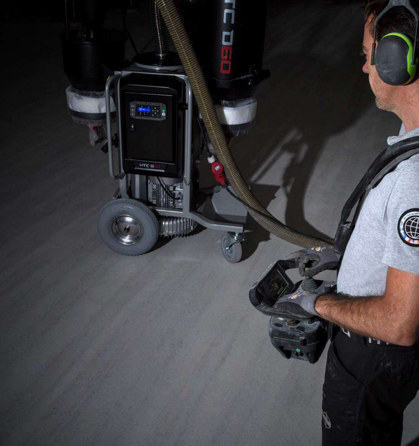
New highly effective filter cleaning function. Easy operation with two buttons.
