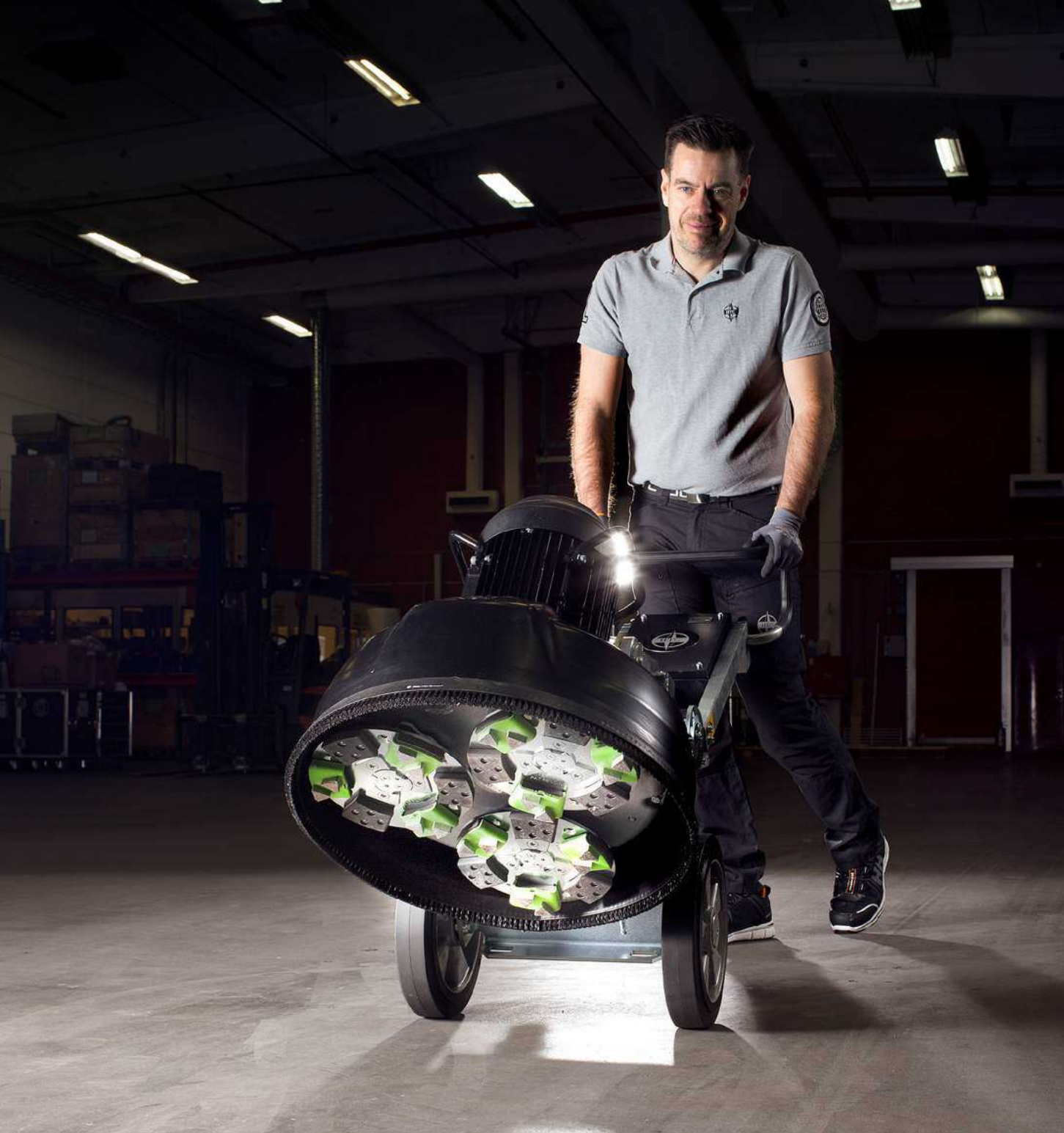
The grinding head on the HTC 510 has a unique design, built to keep out dust and moisture.
